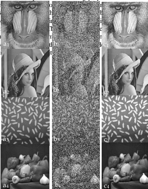
Fig.4 Subjective performance illustration of proposed filtering algorithm for Baboon, Lena, Rice and Pepper images:(a 1,2 & 3 )noise free image (b 1,2,& 3 ) Lena image corrupted with 50% impulse noise, (c 1,2 & 3 ) proposed filtered images.
